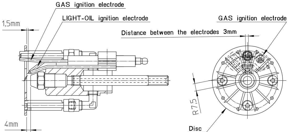
SCHEME OF POSITIONING ELECTRODES LIGHTING GM X3
