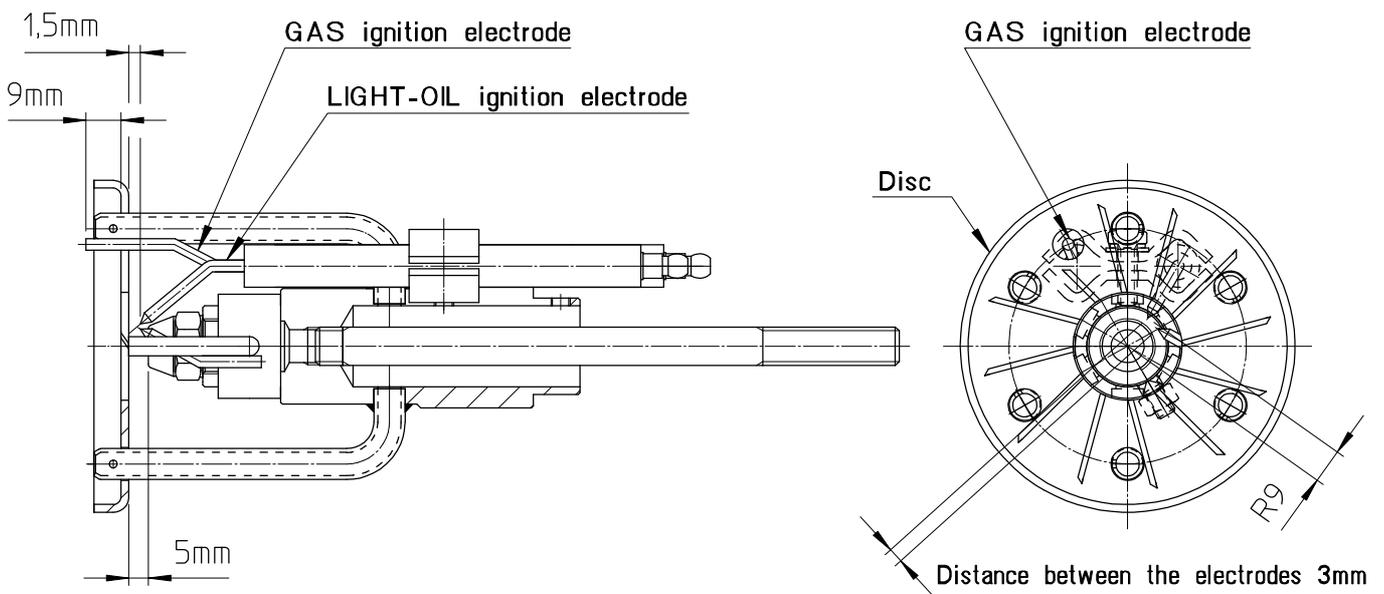
SCHEME OF POSITIONING ELECTRODES LIGHTING GM X4
